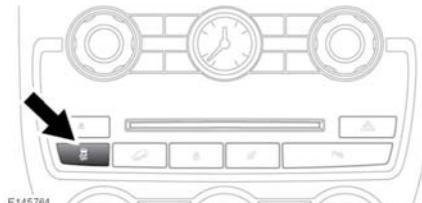
To disable DSC, press and briefly hold the DSC OFF switch on the fascia. The DSC off warning lamp will illuminate continuously. See **35, DYNAMIC STABILITY CONTROL (DSC) OFF (AMBER)**. Deactivating DSC also reduces the level of Traction control intervention and may lead to an increase in wheel spin.
