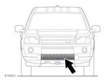
Make sure the areas around air intakes and the front grille are clean and clear of debris. Pay particular attention to the lower grille and radiator. Failure to do so may cause the engine to overheat, leading to severe engine damage.
