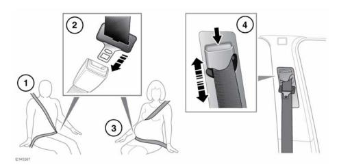
PUTTING ON A SEAT BELT: Draw the belt out smoothly and make sure the belt height, the seat and your position on the seat, are correct.
