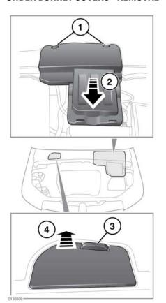
1. Press the tabs to release the cover from the casing.
