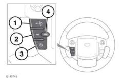
SET+: Press to set the speed or to increase the set speed. The Cruise control warning lamp will illuminate to confirm that Cruise control is operational. See 37, CRUISE CONTROL (GREEN).
