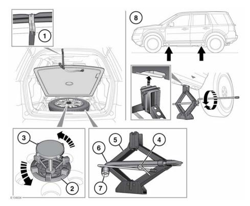
The spare wheel is heavy and if handled incorrectly may cause injury. Use extreme caution when lifting or manoeuvring the wheels.
