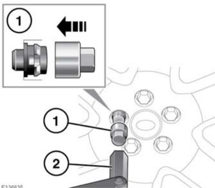
1. Insert the adaptor into the locking wheel nut, making sure that it is fully engaged.
