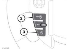
Hill Descent Control (HDC) is designed to restrict vehicle speed to a set limit when travelling downhill.
