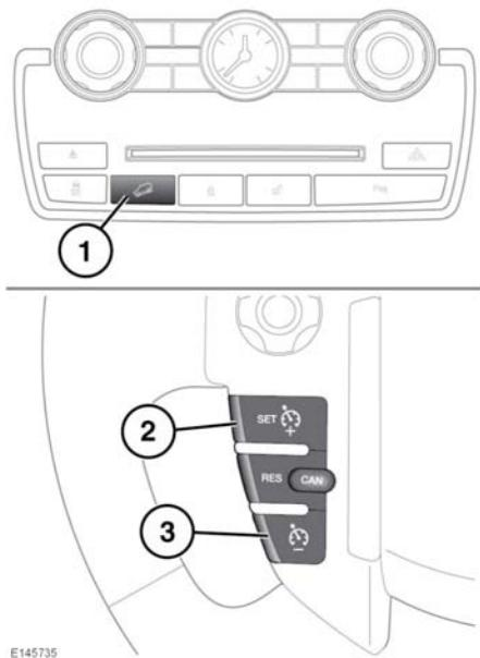
Hill Descent Control (HDC) is designed to restrict vehicle speed to a set limit when travelling downhill.
