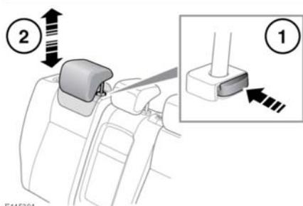
1. Press the locking collar to release the head restraint.
