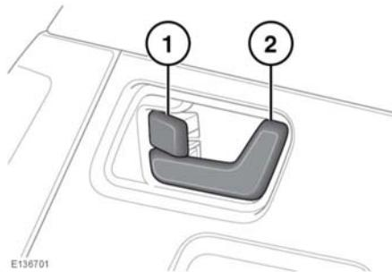
From inside the vehicle, all of the doors can be locked by pressing either the driver or passenger lock lever (1).
