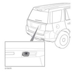
When Reverse (**R**) gear is selected, the screen automatically displays a wide angle, colour image from the rear of your vehicle.
