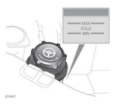
The level of fluid can be seen through the translucent body of the reservoir.
