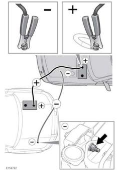
Switch off all electrical equipment before following this procedure. All electrical equipment must remain switched off until the procedure is complete.
