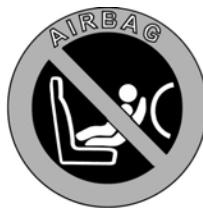
This symbol, affixed to the end of the fascia on the passenger side, warns against the use of a rear-facing child seat in the front passenger seat, when a front passenger airbag is fitted and operational.
