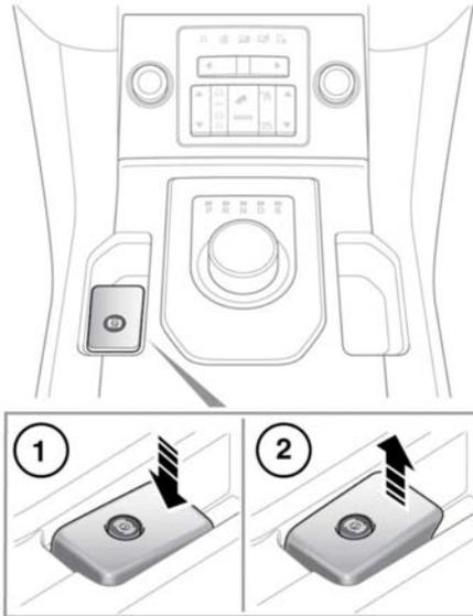
The switch which operates the EPB is mounted on the center console, to the side of the gear selector.
