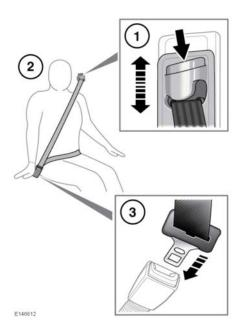
1. **Seat belt height adjustment:** Press to release the catch.
