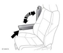
If fitted, the folding armrest may be stowed by moving to the vertical position. Use the adjuster wheel (arrowed) to set the required height.
