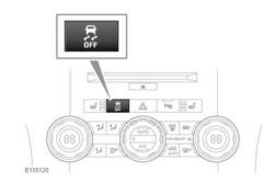
To disable DSC, press and briefly hold the DSC OFF switch on the facia (the DSC off warning lamp will illuminate continuously). Deactivating DSC also reduces the level of Traction control intervention and may lead to an increase in wheel spin. See 52, DYNAMIC STABILITY CONTROL (DSC) (AMBER).
