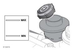
The level of fluid can be seen through the translucent body of the reservoir.
