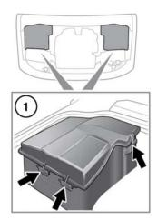
1. Press the tabs to release the cover from the casing.
