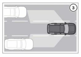
The Blind Spot Monitor (BSM) system monitors an area adjacent to your vehicle, that is not easily visible to the driver. The system is designed to identify any road user passing your vehicle (3) that is within this blind spot, while disregarding other objects which may be stationary or traveling in the opposite direction.
