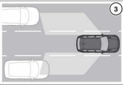
The Blind Spot Monitor (BSM) system monitors an area adjacent to your vehicle, that is not easily visible to the driver. The system is designed to identify any road user overtaking your vehicle (3) that is within this blind spot, while disregarding other objects which may be stationary or traveling in the opposite direction.
