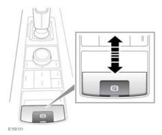
With the ignition turned on, press the brake pedal and press down on the EPB switch. This will release the electronic parking brake.
