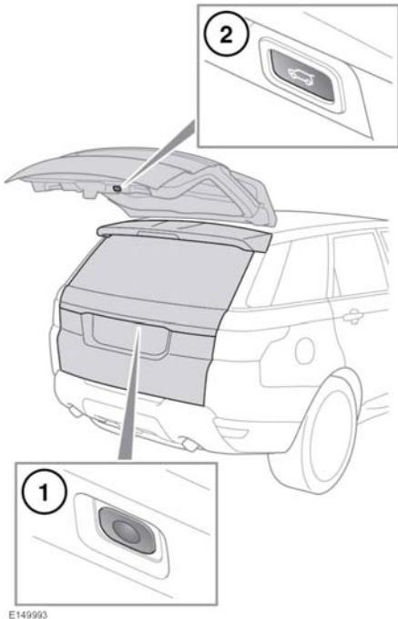
1. Tailgate open/close using the exterior button. Press to open, stop, reverse direction or close the tailgate.
