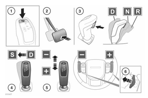
Gear selector status is displayed in the Message centre. See **45**, **INSTRUMENT PANEL**. Also the appropriate LED indicator, on top of the gear selector, will illuminate to confirm selection.
