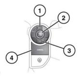
SET+: Press to set the speed or to increase the set speed. The cruise control indicator illuminate to confirm cruise control is operational (see 52, CRUISE CONTROL (GREEN)).
