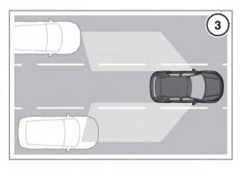
If an object is identified by the system as being an overtaking vehicle/object, an **amber** warning icon (1) illuminates in the relevant exterior mirror, to alert the driver that there is a potential hazard in the vehicle's blind spot and therefore, that a lane change might be dangerous.
