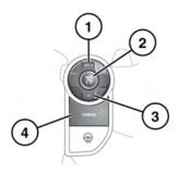
SET+: Press to set the speed or to increase the set speed. The cruise control warning lamp will illuminate to confirm cruise control is operational (see 62, CRUISE CONTROL (GREEN)).
