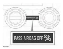
The system will adjust the passenger air bag status and operate the status indicator as follows:
