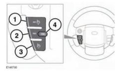
SET+: Press to set the speed or to increase the set speed. The cruise control warning lamp will illuminate to confirm cruise control is operational (see 60, CRUISE CONTROL (GREEN)).
