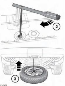
Place the wheel under the vehicle with the styled face uppermost.
