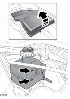
The right hand under-hood cover (as viewed from the front of the vehicle) must be removed to check the brake fluid level, See **160, UNDER HOOD COVERS - REMOVAL**.
