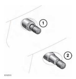
Wheels fitted with TPMS can be visually identified by the external metal lock nut and valve (1). All Land Rover non-TPMS wheels have a rubber valve fitted (2).
