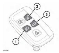
To raise the vehicle press and hold button (1) and button (2) together.
