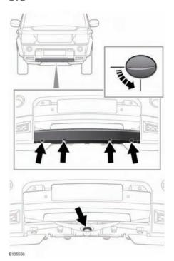
The front towing point is located behind a removable cover in the lower front bumper.
