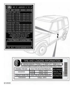
The recommended tire pressures are listed on a label located in the driver's door opening.
