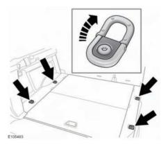
To assist in safely securing large items of luggage, four fixing points are located in the rear loadspace floor.
