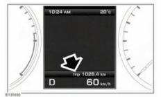
A short press (1 second or less) or a series of short presses of the **i** button will change the trip computer display.
