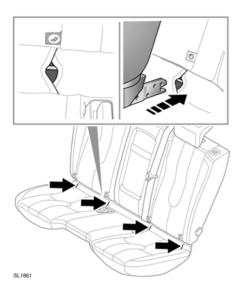
LATCH anchorage child restraints can be fitted only to the outer seat positions on the second row of seats.
