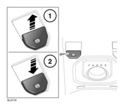
To apply the parking brake while the ignition is on or off, with the vehicle stationary, pull up the lever and release it.
