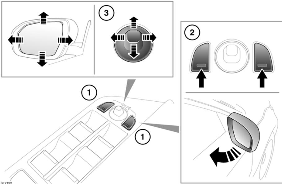
1. Mirror selector switches. Press to select the left or right mirror.
