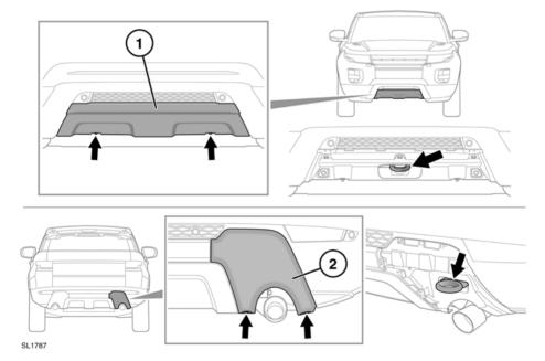
The towing points are located behind panels in the bumpers. Panel design will vary depending on the vehicle specification. To access the towing points:
