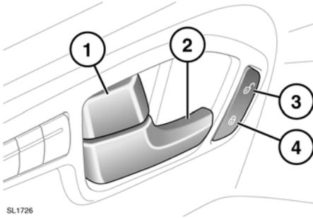
1. Press a locking lever to lock a door. Pull the lever back to unlock. Operating either front door locking levers will lock or unlock all doors.
