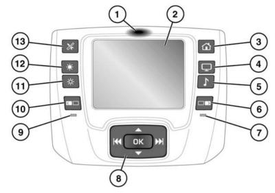
**Note:** The rear media remote control communicates via infra-red and must be pointed towards the receiver in the rear screen.
