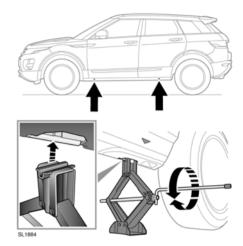
1. Locate the jack under the relevant jacking point.
