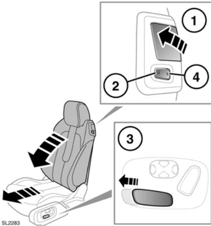
1. Lift the locking lever (1) and pivot the seatback forwards.
