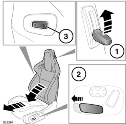
1. Lift the locking lever (1) and pivot the seatback forwards.
