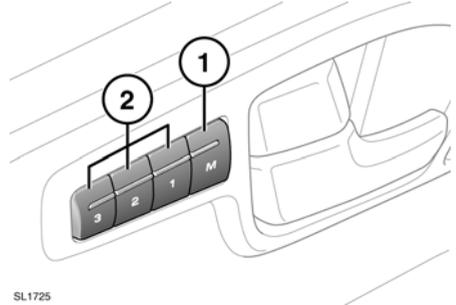
1. On the driver's door, press the memory store button to activate the memory function. The switch indicator will illuminate.
