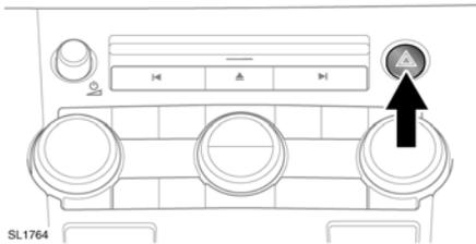
Press to turn the hazard warning lamps on. Press again to turn off. When the hazard warning lamps are operating, the direction indicator warning lamps will flash in time with the hazard warning lamps.
