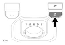
To disable DSC, press and briefly hold the DSC OFF switch. The DSC OFF warning lamp will illuminate continuously. The amber DSC OFF warning lamp in the instrument panel will also illuminate. See 70, DYNAMIC STABILITY CONTROL (DSC) (AMBER). Deactivating DSC also reduces the level of electronic traction control intervention and may lead to an increase in wheel spin.
