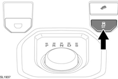
To disable DSC, press and briefly hold the DSC OFF switch. The DSC OFF warning lamp will illuminate continuously. The amber DSC OFF warning lamp in the instrument panel will also illuminate. See **70, DYNAMIC STABILITY CONTROL (DSC) (AMBER)**. Deactivating DSC also reduces the level of electronic traction control intervention and may lead to an increase in wheel spin.
